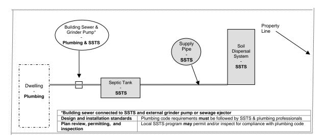
Scenario 4: Single family dwelling on an individual lot with an SSTS with or without an outside grinder pump or sewage ejector, in areas of the state that **do** locally enforce the plumbing code.
