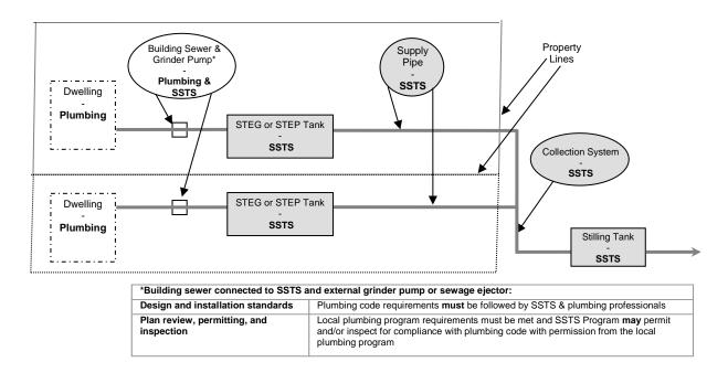
Scenario 8: Individual dwellings on multiple lots with or without an outside grinder pump or sewage ejector served by gravity or pressure sewer to a publically owned treatment works (POTW) in any area of the state.
