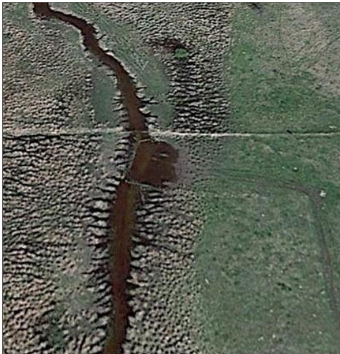
Photo 6. Cattle trampling along Darrigan's Creek, showing the well-documented channel changes of becoming wider and shallower where cattle traverse the banks. Note also the many gullies on the bank from cattle hooves and subsequent erosion.
