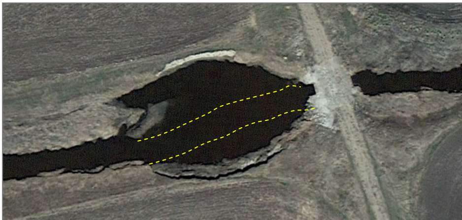
Photo 10. This culvert on AUID-502 (along CSAH-2) is undersized, and during times of higher flow volumes, it constricts flow, increasing the velocity and erosive forces of the water as it exits the culvert, causing a large scour pool. The banks of this pool are raw and steep, and the southern bank has eroded right up to the edge of the cultivated field surface. Many truckloads of soil have eroded from this scoured area. The yellow dotted lines delineate the width of the channel as it should be here.
