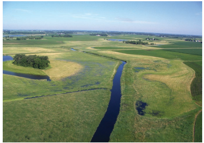
The straightened stream bed of High Island Creek is characteristic of the altered hydrology prevalent in the watershed.
