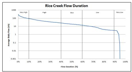
Figure 7.1 Flow duration curve for Rice Creek.
