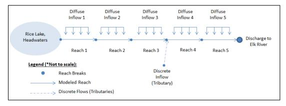
Figure 6-1 - Rice Creek Model Schematic Diagram
