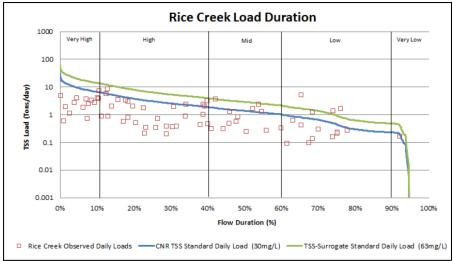
Figure 7.2 TSS Load duration curve for Rice Creek
