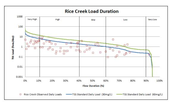
Figure 7-2 - TSS Load duration curve and necessary TSS reductions
