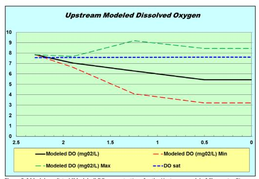
Figure 3.4 Model-predicted (Modeled) DO concentrations for the Upstream model of Clearwater River
