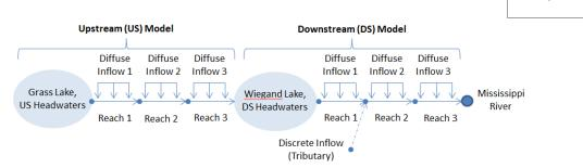
Figure 6-3 - Clearwater River Watershed Model Schematic Diagram
