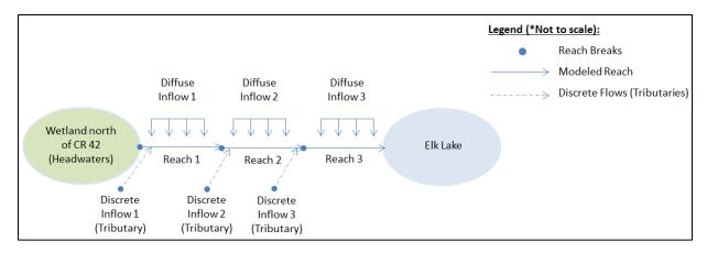
Figure 6-2 - Battle Brook Model Schematic Diagram
