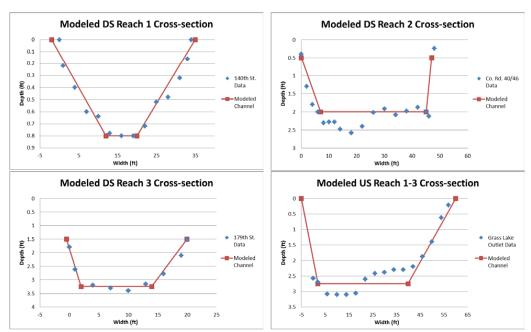
Figure 3.1 Reach cross-section tape-down data and trapezoidal channel approximation for downstream reach.
