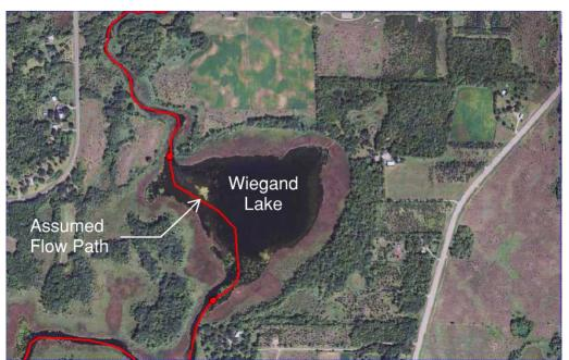
Figure 3.5 Clearwater River short-circuiting Wiegand Lake
