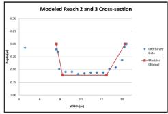
Figure 3.1 Reach cross-section survey data and trapezoidal approximation for reaches 1, 2, and 3.
