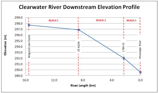
Figure 2.1 MN LiDAR elevations used to estimate reach slopes for Clearwater River Downstream model
