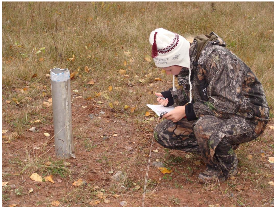
Figure 3. Measuring infiltration rate using MPD infiltrometer on a ski slope (October 2009)
