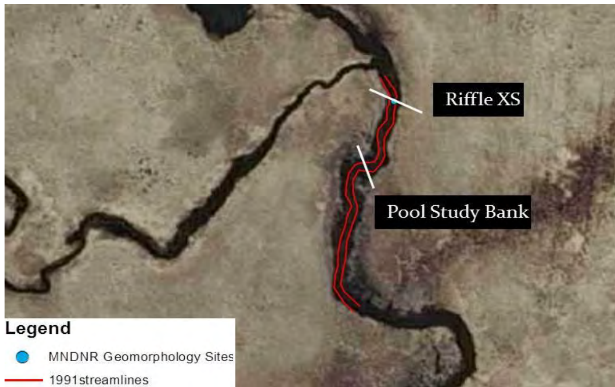
Figure 31. Aerial photo of the survey reach with labeled cross section locations and 1991 stream lines.
