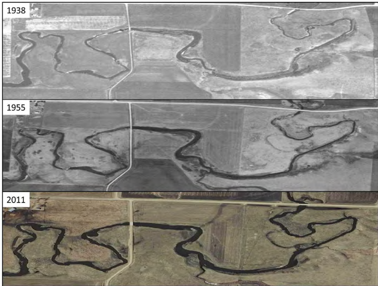
Figure 50. Aerial photo imagery from 1938-2011 of Flandreau Creek. The pattern of the channel is very similar in 1938 to what it is presently, and some areas appear to be narrower in the past, while others remain similar.
