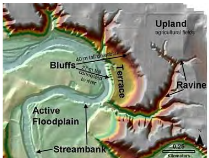
Figure 5. Digital elevation model of a portion of the Le Sueur River watershed, showing the primary sources of sediment.
