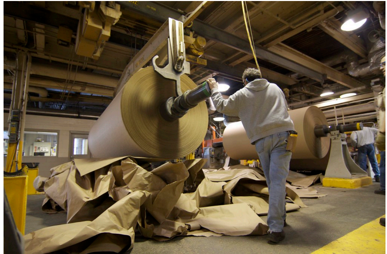
Making new kraft paper from recycled paper at WestRock in St. Paul
